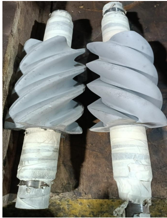
Shot Blasting of the rotors
